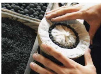
Each shell is carefully packed with powder by hand, one slot at a time.
