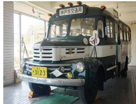
Cab-behind-engine type bus that exists at present
