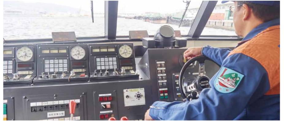
Inside the fourth fireboat Tachibana: the center levers are for operating the water cannon and the pump.
